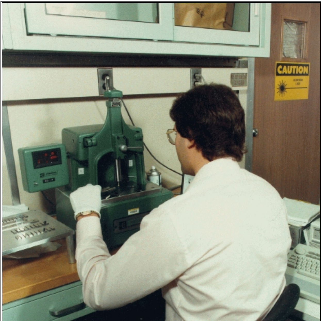
Figure 7.14-1 Calibration and Measurement of Gage Blocks by Mechanical Intercomparison in Progress
