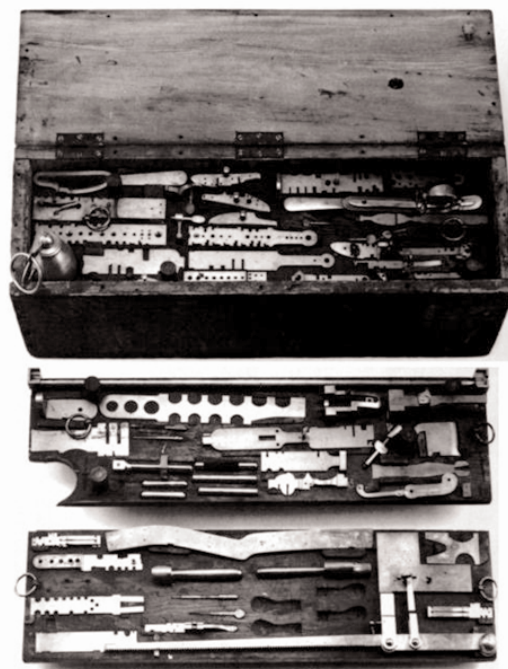
Fig. 2. One complete set of gauges used in the manufacture of a single model pistol.
